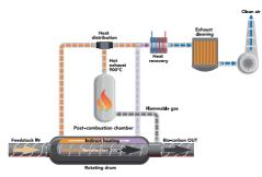
The gases produced during torrefaction are burned and the generated energy is used to heat a rotary drum. Therefore the system is self-sustaining.
